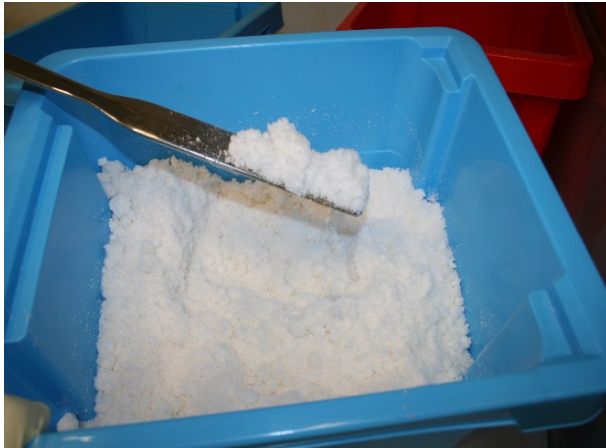
Fig, 21. Solidification of Organic-Methanol-Ethanol with Tritium
